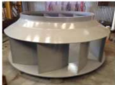
Application of primer by hand due to complexity
