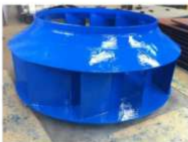
View of impeller completion
